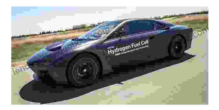
Fuel cell vehicles (FCVs) represent a futuristic approach to sustainable transportation, offering the promise of zero-emission driving. Fueled by hydrogen, FCVs generate electricity through an electrochemical reaction between hydrogen and oxygen, propelling the vehicle with an electric motor while emitting only water vapor as a byproduct.
